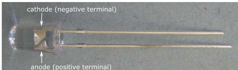
Figure 9-9: The cathode (negative side) of a typical single-color LED is attached to the larger metal plate inside the plastic housing and to the shorter lead (until you clip the leads).
