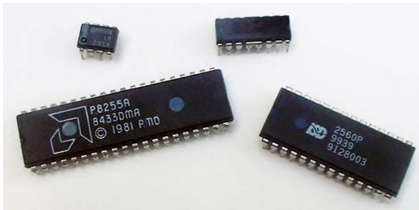
Figure 11-6: A popular form of integrated circuit is the dual in-line package (DIP).
