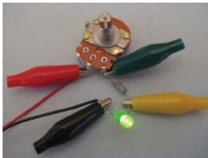
Figure 5-14: A resistor in series with a potentiometer ensures that current to the LED is restricted even if the pot is dialed down to zero ohms. Without that resistor, the LED is toast.
