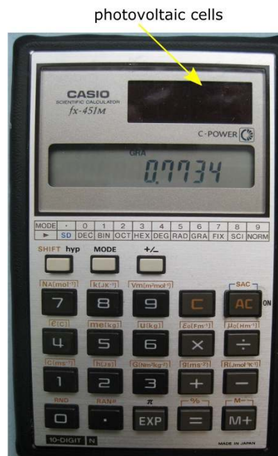
Figure 1-8: This calculator is powered by photovoltaic cells.
