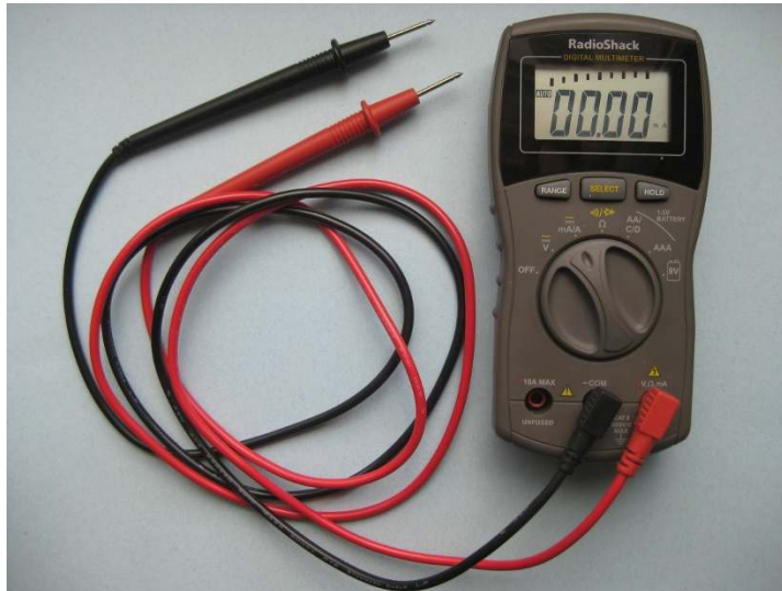
Figure 16-1: Multimeters measure voltage, resistance, current, and continuity.
