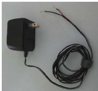
Figure 12-6: This AC adapter converts 120 volts AC to 7.5 volts DC and supplies up to 300 mA of current. I modified the output of this adapter to make it easier to use in DC circuits.
