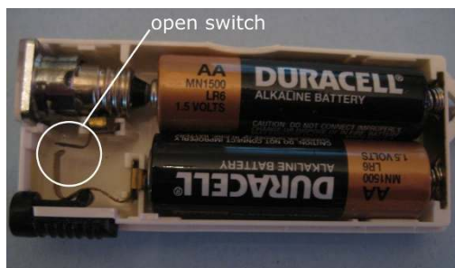
Figure 3-2: A switch in the open position disconnects the light bulb from the battery, creating an open circuit.
