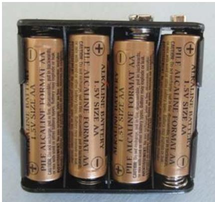
Figure 12-5: Four 1.5 volt batteries in a battery holder produce about 6 volts across the red and black leads.
