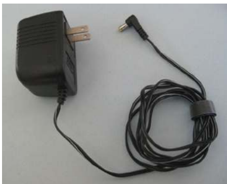
Figure 12-6: This AC adapter converts 120 volts AC to 7.5 volts DC and supplies up to 300 mA of current. I modified the output of this adapter to make it easier to use in DC circuits.
