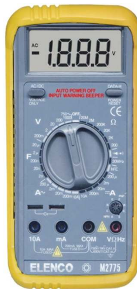
Figure 13-1: Multimeters measure voltage, resistance, and current.
