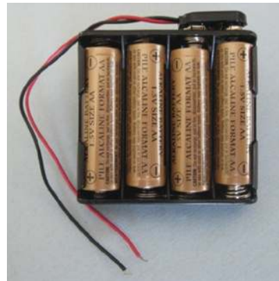
Figure 12-5: Four 1.5 volt batteries in a battery holder produce about 6 volts across the red and black leads.
