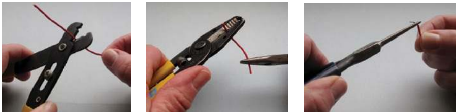
Figure 15-5: Cutting, stripping, and bending an interconnect wire.
